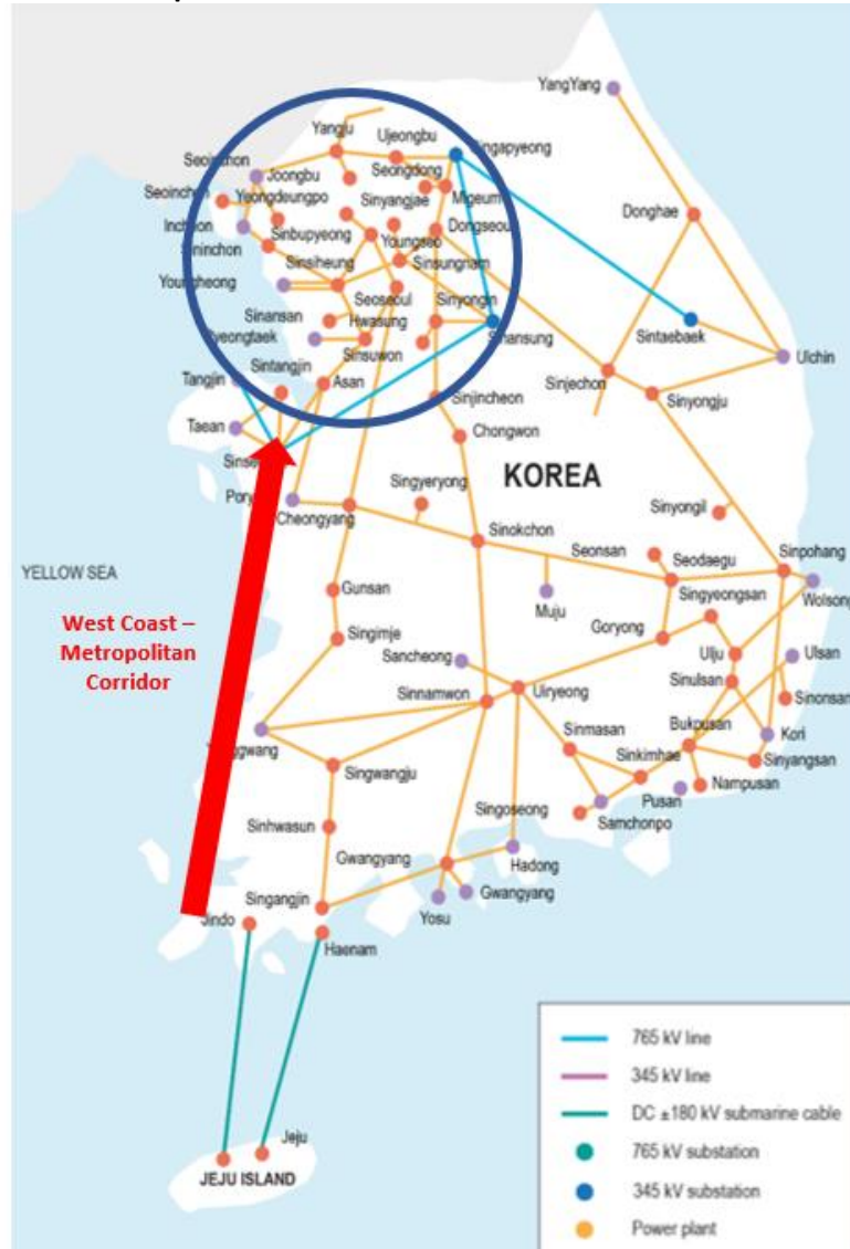
Chart 14: South Korea Map of Transmission Power Grid with Vision of New Corridor Added
